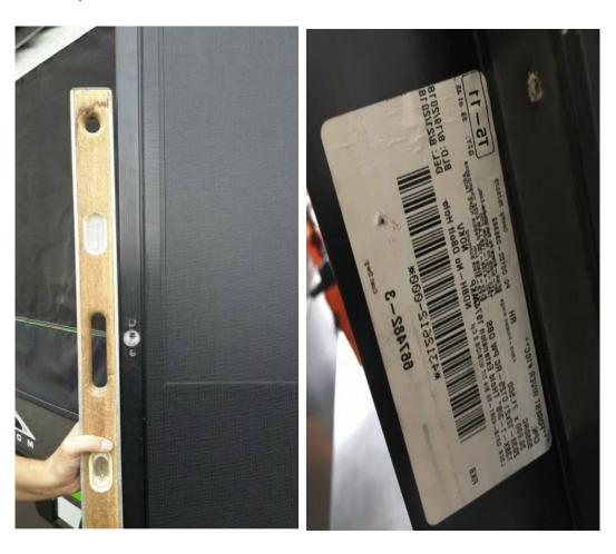
• **Compartment door**- If the door is bowed, we require a picture of a straight edge for us to see the defect. We also require a picture of the complete door and the tag on the inside of the compartment door.
